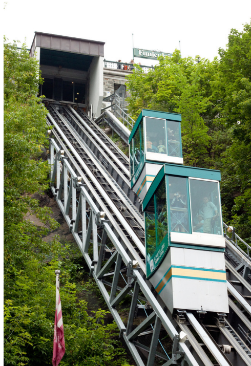
Community-Scale Cable Cars consist of both top-supported and bottom-supported transport systems where vehicles are propelled by a steel cable. Examples in the above photos include systems built in Quebec City (left), Switzerland (top right) and La Paz (bottom right).
