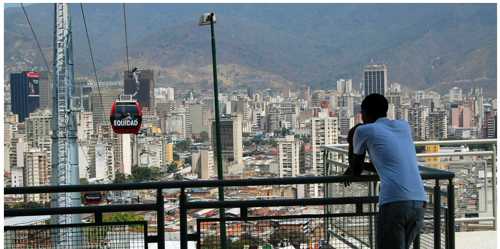
Doppelmayr supplied the electro-mechanical equipment for the Caracas, Metrocable. The first Caracas Metrocable is 5 stations long with a little more than a mile in length. It connects directly to the Metro/ subway and allows residents living in isolated hilltop communities access to wider transportation options.
