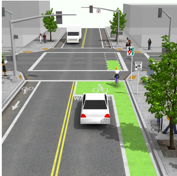
Example of an intersection Bicycle Box Image: NACTO Urban Bikeway Design Guide
