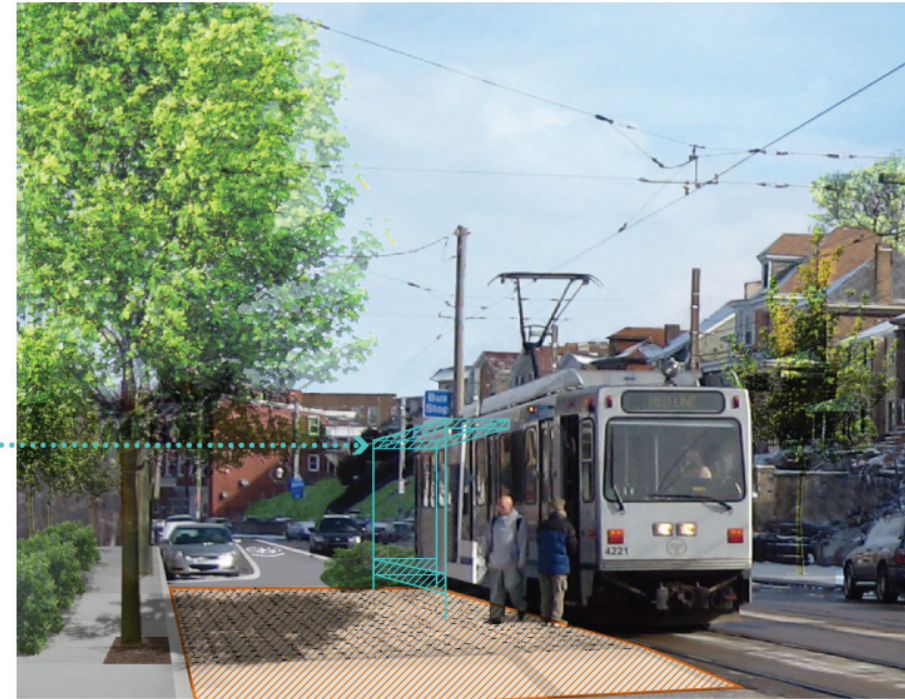
Existing roadway and T platform on Broadway; proposed speed table to connect the sidewalk with the transit stop
